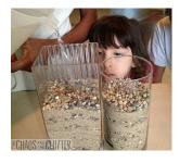
Step 1: In each of the glass containers, layer sand and gravel alternating between the two until they are about  $\frac{3}{4}$  of the way full. This will create an aquifer. An aquifer is the layers of rock, soil and sand that contain water.
