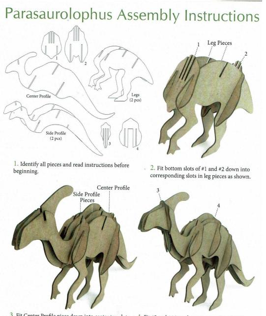
3. Fit Center Profile piece down into center top slots 4. Fit #3 and #4 into the corresponding slots in in #1 and #2. Fit Side Profile pieces down into side top profile pieces as shown. You're done! slots in #1 and #2 as shown.
